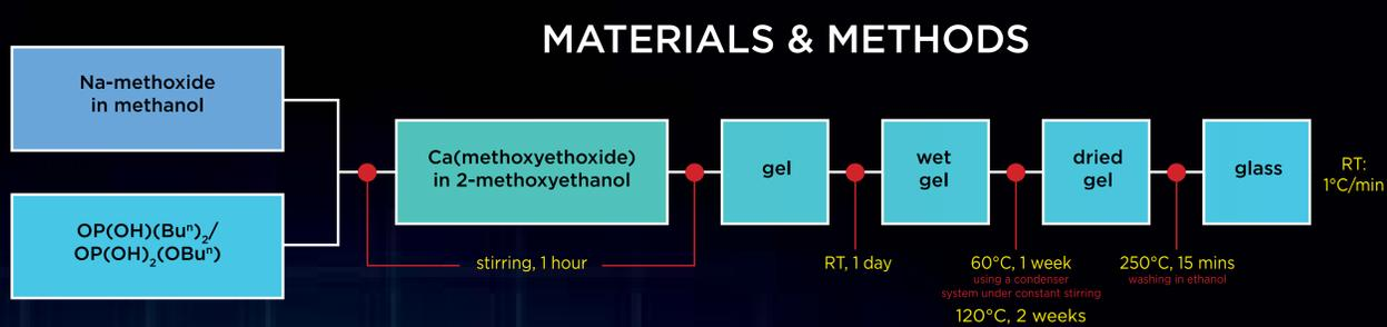
**Fig.1** Flow diagram of the sol-gel preparation
